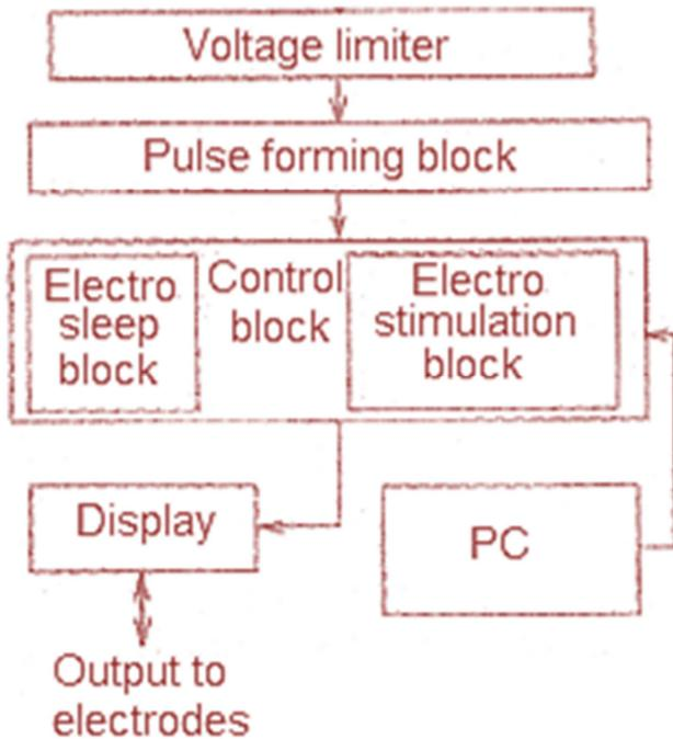
Figure 3. Block diagram of electro stimulation.
